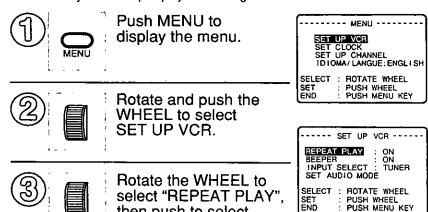
The VCR plays to the end of a tape, or until a blank portion of 30 seconds or more is reached. (Erased portions of tape are not considered blank.) The tape is then automatically rewound and played again and again until Repeat Play is cancelled. All function buttons (REW, FF, etc.) are operational during Repeat Play.
