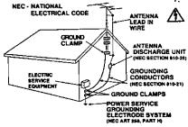
**INSURE SAFE ANTENNA** AND CABLE CONNECTIONS If an outside antenna or cable system is connected to the equipment, be sure the ANTENNA
