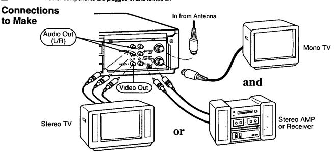
When recording, you may monitor in stereo, by connecting the VCR to either a stereo TV, or a mono sound TV with stereo amp and speakers
